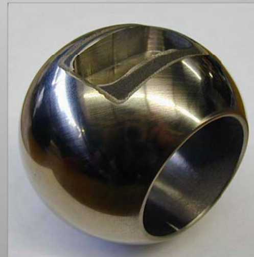
Perrit 01 coated ball DN 2" after lapping
