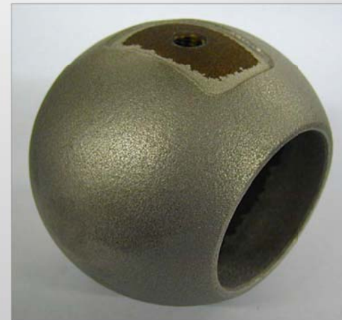
pre machined ball DN 2" after coating with Perrit 01
